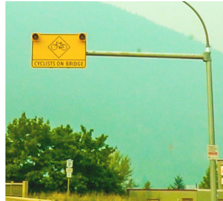
Drivers entering the bridge are notified with a flashing sign when cyclists are currently on the bridge.
