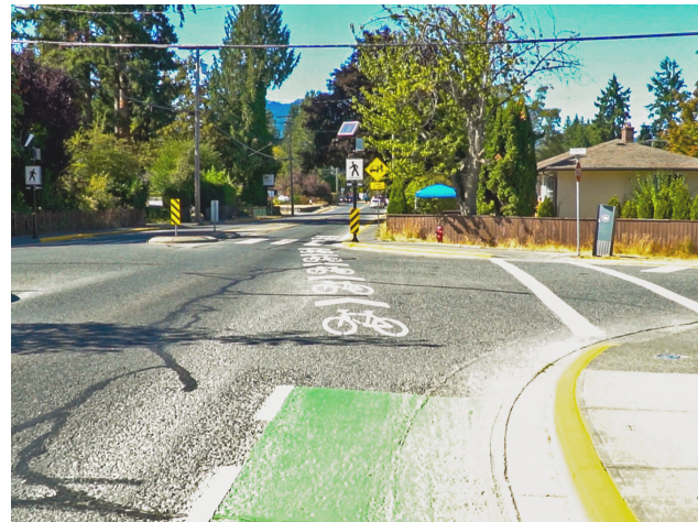
This roadway highlights a bike lane, sidewalk with a yellow line on the outer edge, crosswalk accompanied by a pedestrian crossing sign, and "Share the Road" sign. This shows where the green bike lane ends and moves to a shared road model where the road is too narrow for dedicated bike lane.
